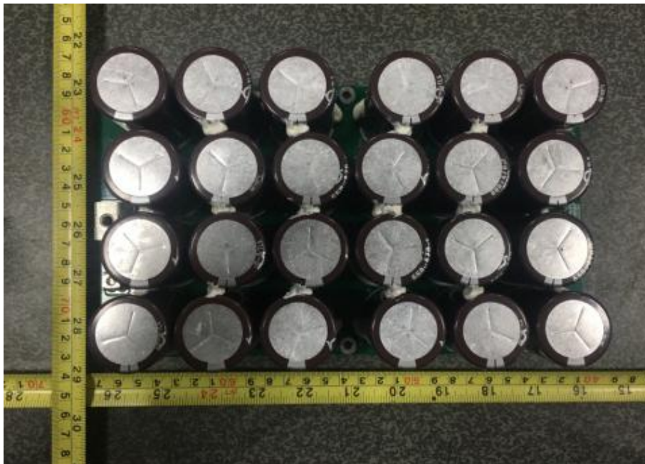
The front of BUS capacitor board
