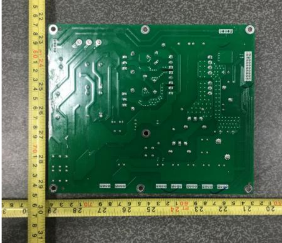
The back of power circuit board
